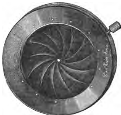
FIG. 10.—Iris Diaphragm, showing a small aperture.
